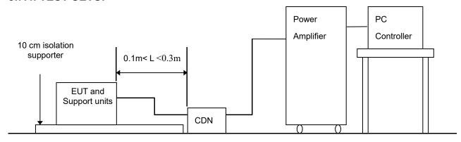
**Note:** 1. The EUT is setup 0.1m above Ground Reference Plane 2. The CDNS and / or EM clamp used for real test depends on ports and cables configuration of
