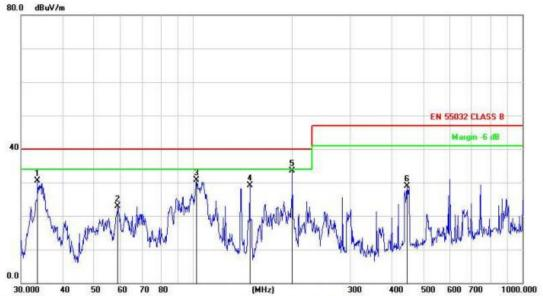
Site LAB Limit: EN 55032 CLASS B Polarization: Vertical Power:
